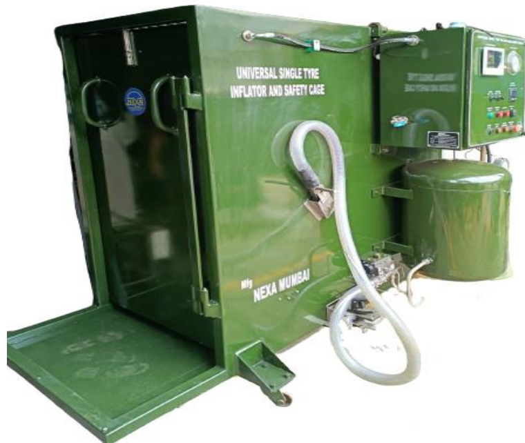
Fig-1: Universal Single Tyre Inflator and Safety Cage
