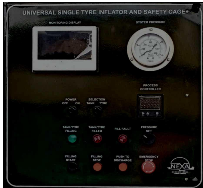
Fig-2: Front Panel of Universal Single Tyre Inflator and Safety Cage
